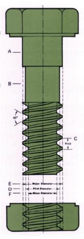
**LEAD:** The distance a screw thread advances axially in one turn.
